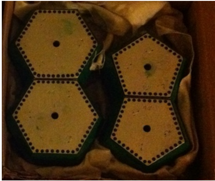
Figure 1: Traditional 2-Hexagon and 2-Pentagon Dies
